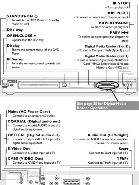
Caution: Do not touch the inner pins of the jacks on the rear panel. Electrostatic discharge may cause permanent damage to the unit.
